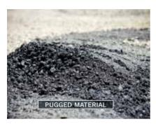
Mixing only ½–1¼ gallons of Activate per ton of screened millings creates a usable paving material that cures in three hours without tracking or raveling. A minimum of 4% residual asphalt cement content is required and a standard pug mill is the recommended method for mixing the solution
